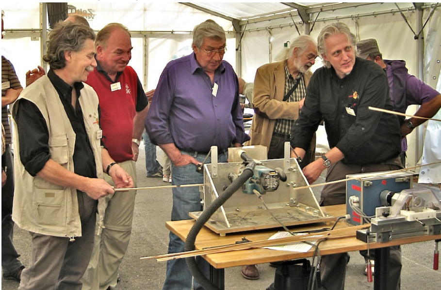
Philipp Sicher (l) and Herbi Kisler (r) rough beveling with a Baginski Beveler under the watchful eyes of Hans-Ruedi Hebeisen (in red) and Wilhelm Aigeldinger (in blue)
